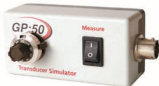
The TST-MV/V simulates the output of any melt pressure transducer, (3.33 mV/V output), adjustment settings for various pressure levels when testing output for existing melt pressure transducers. The simulator is available with standard 6-pin connector or 8-pin (with adaptor cable).
