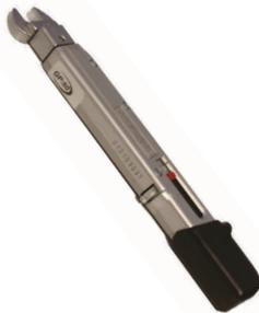
Precision Extrusion Sensor Torque Wrench for the recommended torque of melt pressure and temperature transducers. The TTW-AA is designed to improve transducer accuracy and life expectancy by avoiding unaccounted additional torque to the threads and seat of 1/2-20 UNF transducers, while also eliminating the possibility of side force trauma to the transducer tip area.
