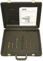
The Hole Machining Tool Kit contains all of the necessary drills and taps to prepare a standard 1/2 - 20 UNF transducer mounting hole. The kit contains the special pilot drill required to machine the 45 degree seat. All tools included in this kit are made of premium grade, high strength tool steel. Care should be taken in the use of proper speeds and feeds, lubricants, and a method to assure continual alignment of each progressing tool.
