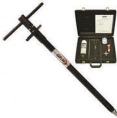
The Cleaning Tool Kit removes unwanted plastic residue from mounting holes before transducer installation. A major cause of damage during installation practices is a transducer installed in a plugged or dirty mounting hole. The Cleaning Tool Kit will give a thorough cleaning of the mounting hole, while also checking the stability of the hole itself. Cleaning tools are available for 1/2-20 and M18 X 1.5 mounting holes.
